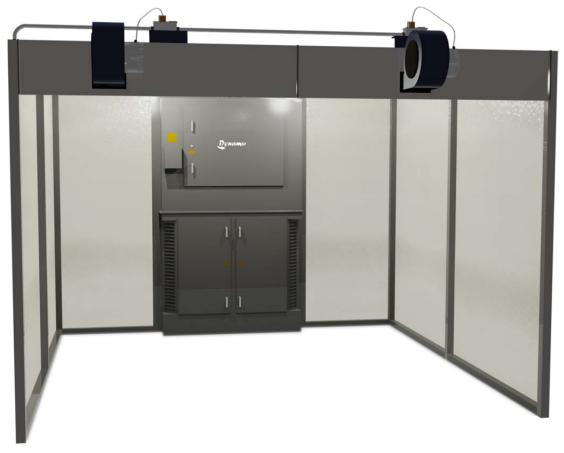
Dynamo dust booths are made for applications where items are too large for a downdraft table. Our dust booths have two standard units. The smaller (9,000 CFM) unit works great in applications using light and medium sanders with light to medium grit paper. The larger (12,500 CFM) model can be used for heavy sanding or even heavy grinding applications done with a very coarse grit paper. This model can be custom made with side openings for use in conjunction with conveyor systems.
